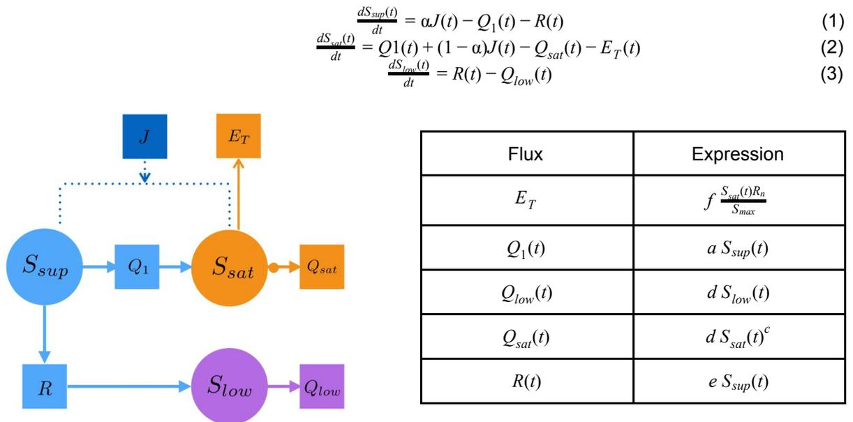
**Figure 1.** EPN of a simple rainfall-runoff model and table of equations to describe fluxes, Rigon et al. (2016b).
