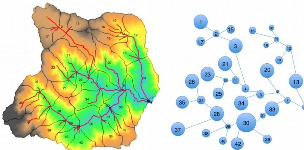
**Figure 2.** Representation of subcatchment connections into NET3 (Bancheri (2017)).
