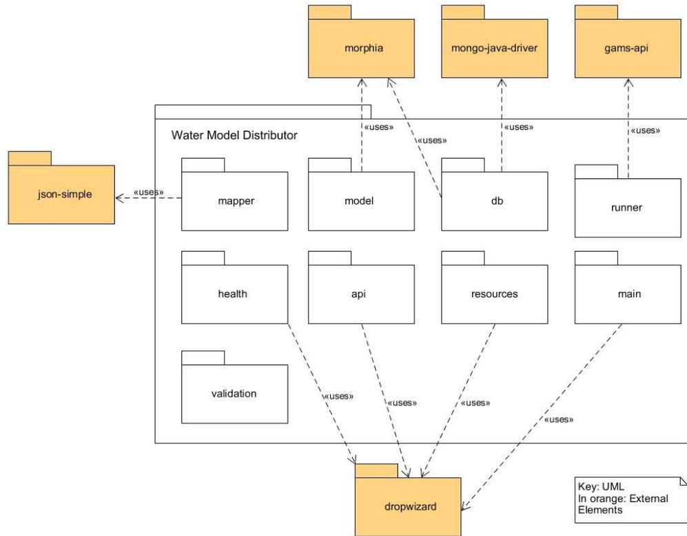
**Figure 2.** Water Model Distributor UML Uses View
