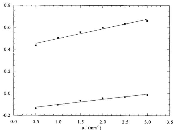
Fig. 5. The slopes,  $m$ , and the intercepts,  $b$ , of the lines shown in Fig. 4 depended linearly on  $\mu'_s$ . The estimate of  $\mu'_s$  obtained from Eq. (5) is used in Eq. (6) to obtain values for  $m$  and  $b$ . These values are then used in Eq. (7) to obtain an estimate for  $g$ . ●,  $m=0.049 \mu'_s - 0.15$ ; ■,  $b=0.089 \mu'_s + 0.41$ .
