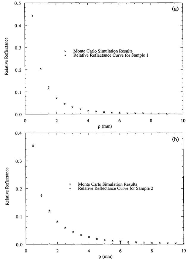
Fig. 6. (a) Comparison of the measured and simulated relative reflectance curves for Sample 1. The optical properties used in the Monte Carlo simulations are  $\mu_s' = 1.15$  and  $g = 0.90$ . (b) Comparison of the measured and simulated relative reflectance curves for Sample 2. The optical properties used in the Monte Carlo simulations are  $\mu_s' = 0.64$  and  $g = 0.84$ .
