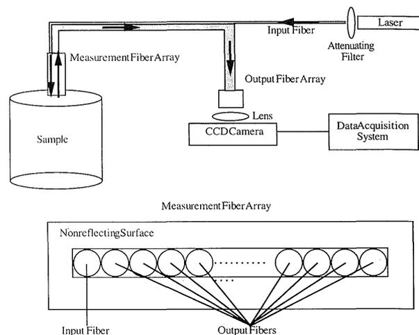
Fig. 2. An array of 25 optical fibers with a diameter of  $500 \mu\text{m}$  is positioned above the sample. Light from a HeNe laser ( $\lambda=632.8 \text{ nm}$ ) is introduced into the sample through the fiber on the end of the array and reflected light is collected by the remaining fibers. After magnification, the intensity of the reflected light collected by each fiber is measured using a CCD camera.
