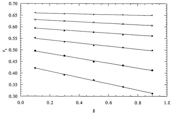
Fig. 4. For a given  $\mu'_s$ , there exists a linear relationship between  $r_1$ , which is the reflectance measured by the output fiber nearest the input fiber and the asymmetry parameter,  $g$ . ●,  $\mu'_s=0.5 \text{ mm}^{-1}$ ; ◆,  $\mu'_s=1.5 \text{ mm}^{-1}$ ; ×,  $\mu'_s=2.5 \text{ mm}^{-1}$ ; ■,  $\mu'_s=1.0 \text{ mm}^{-1}$ ; ▲,  $\mu'_s=2.0 \text{ mm}^{-1}$ ; +,  $\mu'_s=3.0 \text{ mm}^{-1}$ .
