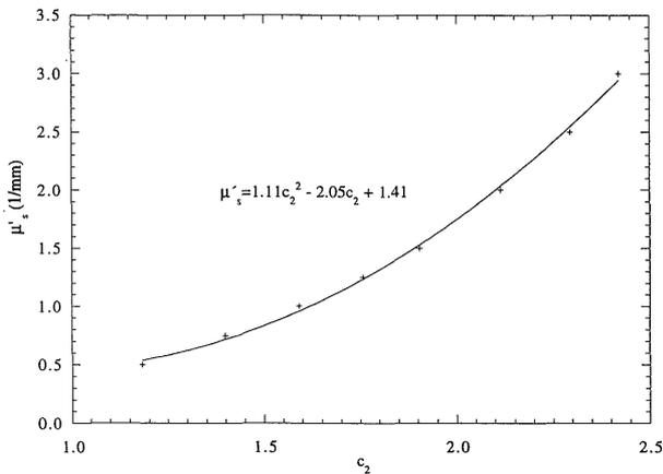
Fig. 3. There exists a quadratic relationship between  $\mu'_s$  and  $c_2$  for the fiber array composed of 500  $\mu\text{m}$  fibers. A value for  $c_2$  is obtained by fitting Eq. (4) to the measured reflectance pattern, and Eq. (5) is then used to obtain an initial estimate for  $\mu'_s$ .
