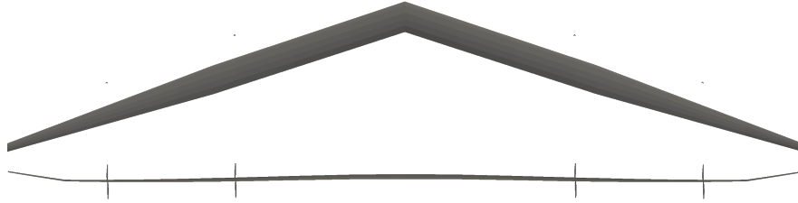
Fig. 7 Top and rear view of the optimal swept flying wing aircraft design during design operation.
