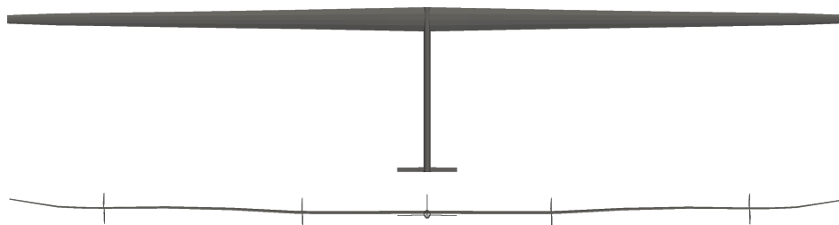
Fig. 8 Top and rear view of the optimized single boom solar aircraft design during design operation.
