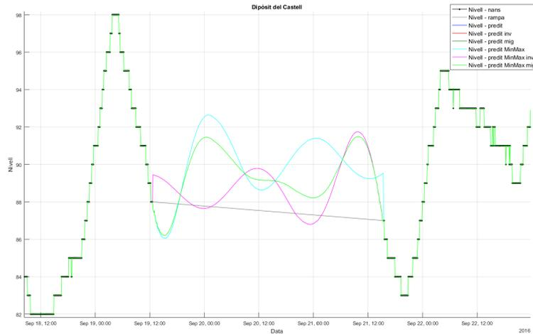
Figure 2 Reconstruction of a lost data stream.
