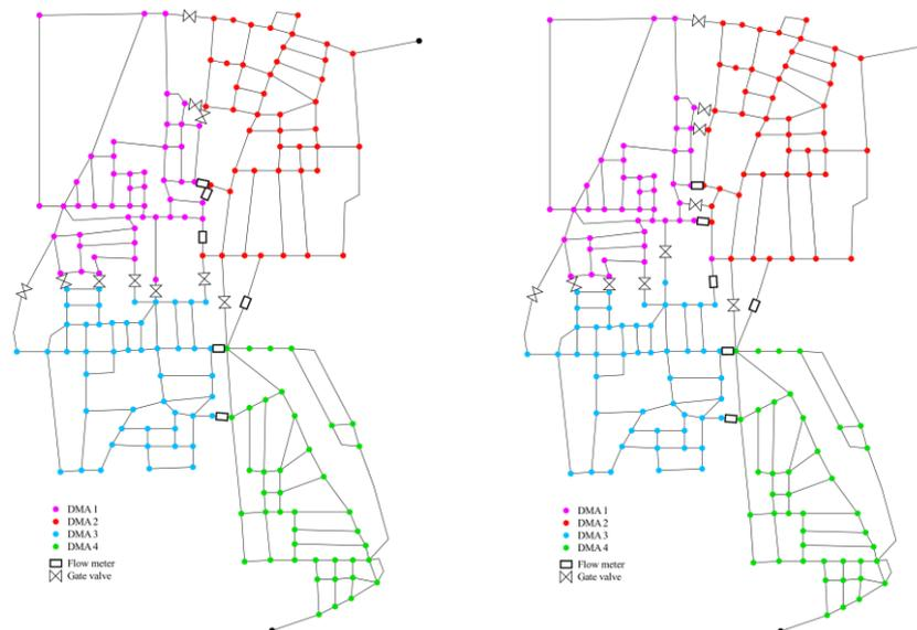
**Figure 3.** Comparison between a)  $nR$ -WNP and b)  $R$ -WNP layouts
