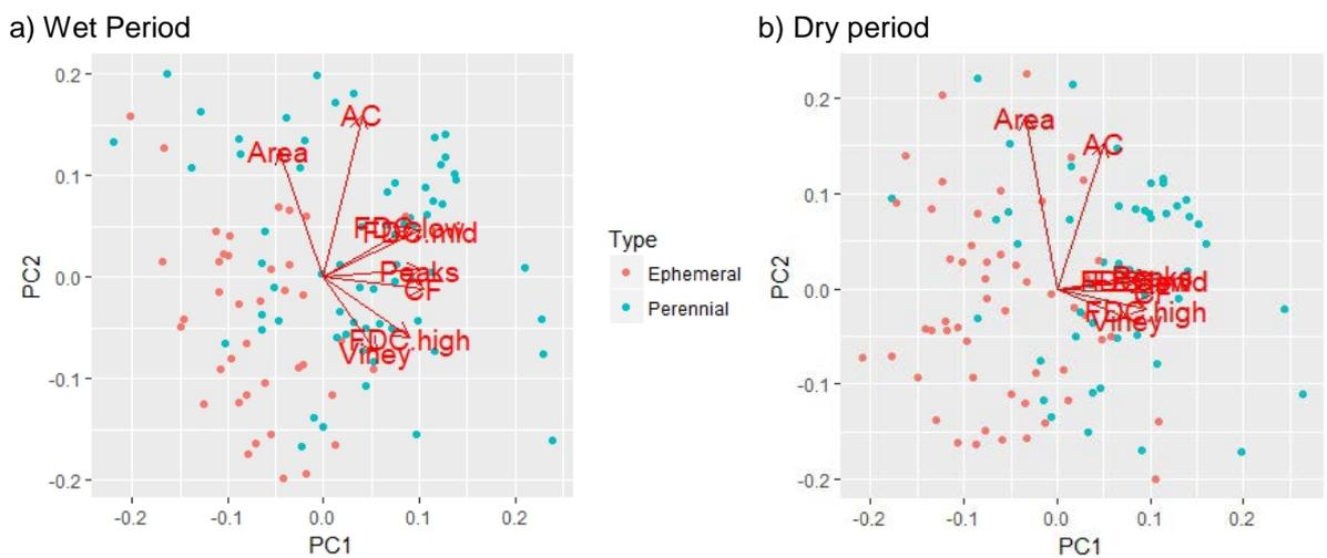
**Figure 3.** Biplots of the catchment characteristics in the: a) wet and b) dry period. The PCs are plotted against river type. Perennial is classified as no flow  $\leq$  1% of the time and Ephemeral is classified as no flow  $>$  1% of the time.
