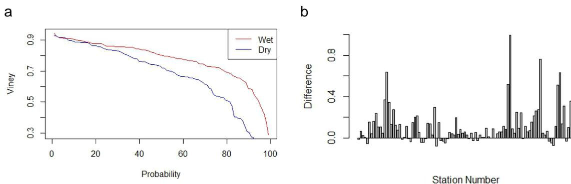
**Figure 2.** a) Exceedance probability of the Viney objective function value for both wet and dry periods for all catchments b) Difference in objective function values between the wet and dry periods (wet – dry).
