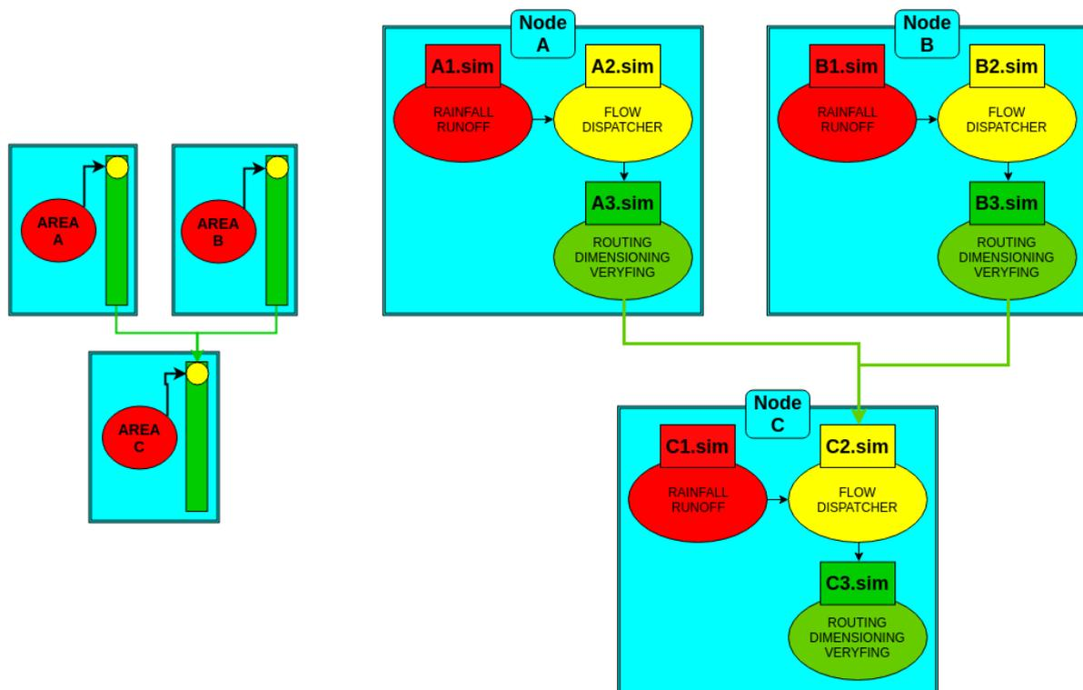
**Figure 1.** Example scheme of a three node physical problem (on the left) and its correspondent implementation in JSWMM (on the right)
