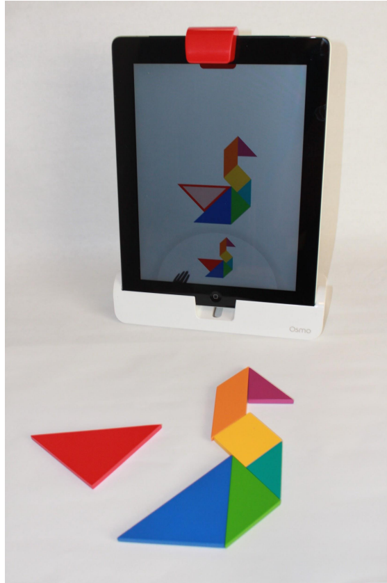
Figure 5. The OSMO interface, in which the controls are manipulatives detected by a downward-looking camera.
