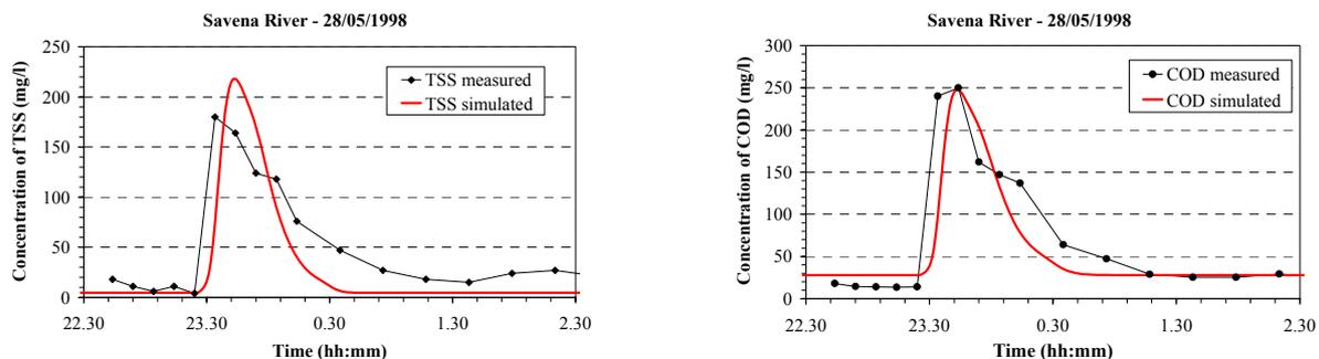
*Comparison between simulated and measured TSS and COD in the Savena river (about 300 meters downstream the overflow) on May 28<sup>th</sup>, 1998.*
