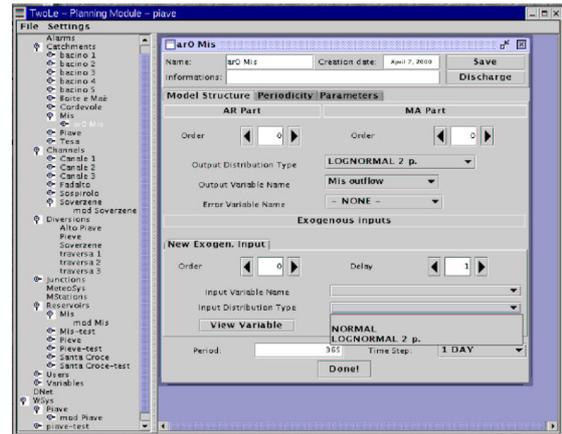
Figure 9: The TwoLe GUI: calibration of an ARMA.
