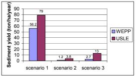
Figure 5. Sediment yield at the bottom of a slope using the WEPP and USLE
