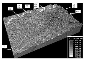
Figure 6. Digital elevation model (DEM) of the Bodong site with erosion 'hot spots' for USLE (U) and GUEST (G) for scenario 1
