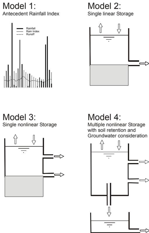
**Figure 1:** Scheme of the applied model types.
