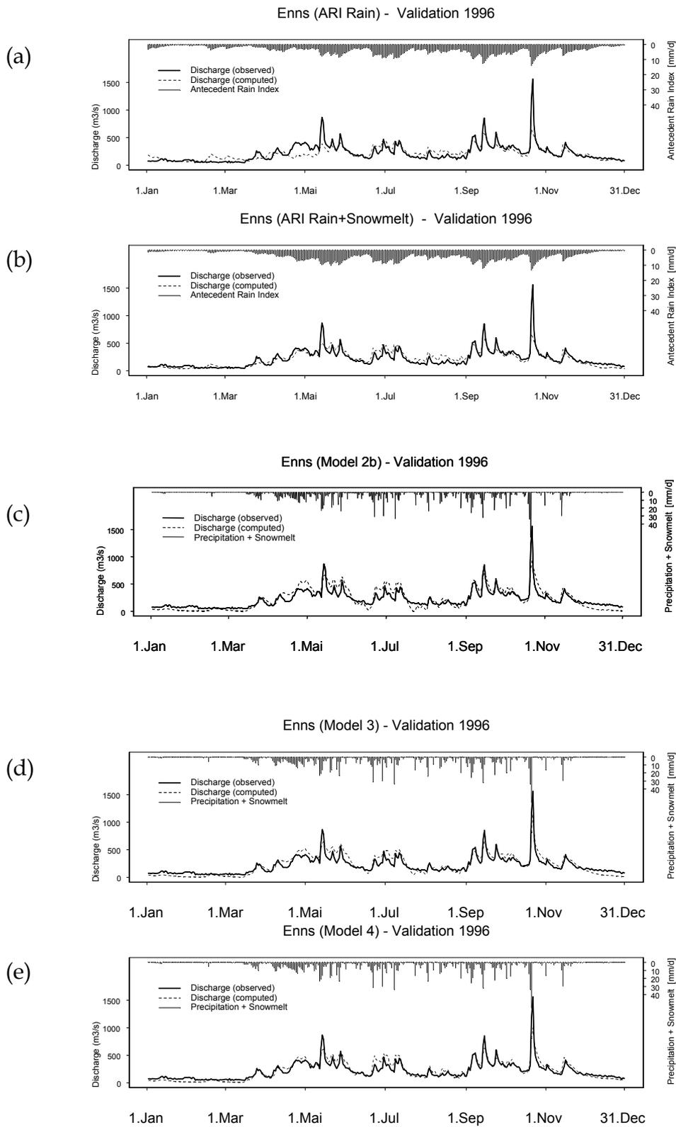
**Figure 2:** Validation performance of (a) Model 1a (ARI Rain), (b) Model 1b (ARI Rain+Snowmelt), (c) Model 2b (Single Storage + Soil Reservoir), (d) Model 3 (Single storage - double outflow), (e) Model 4 (Double storage - double outflow).
