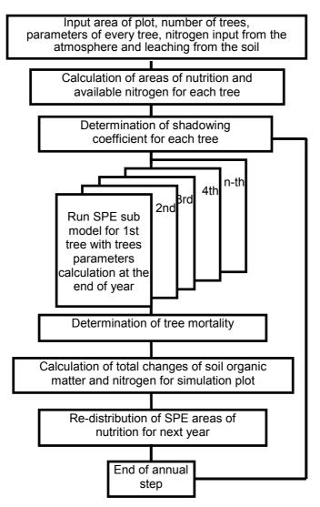
Figure 1. Flow-chart of year step of the EFIMOD model.
