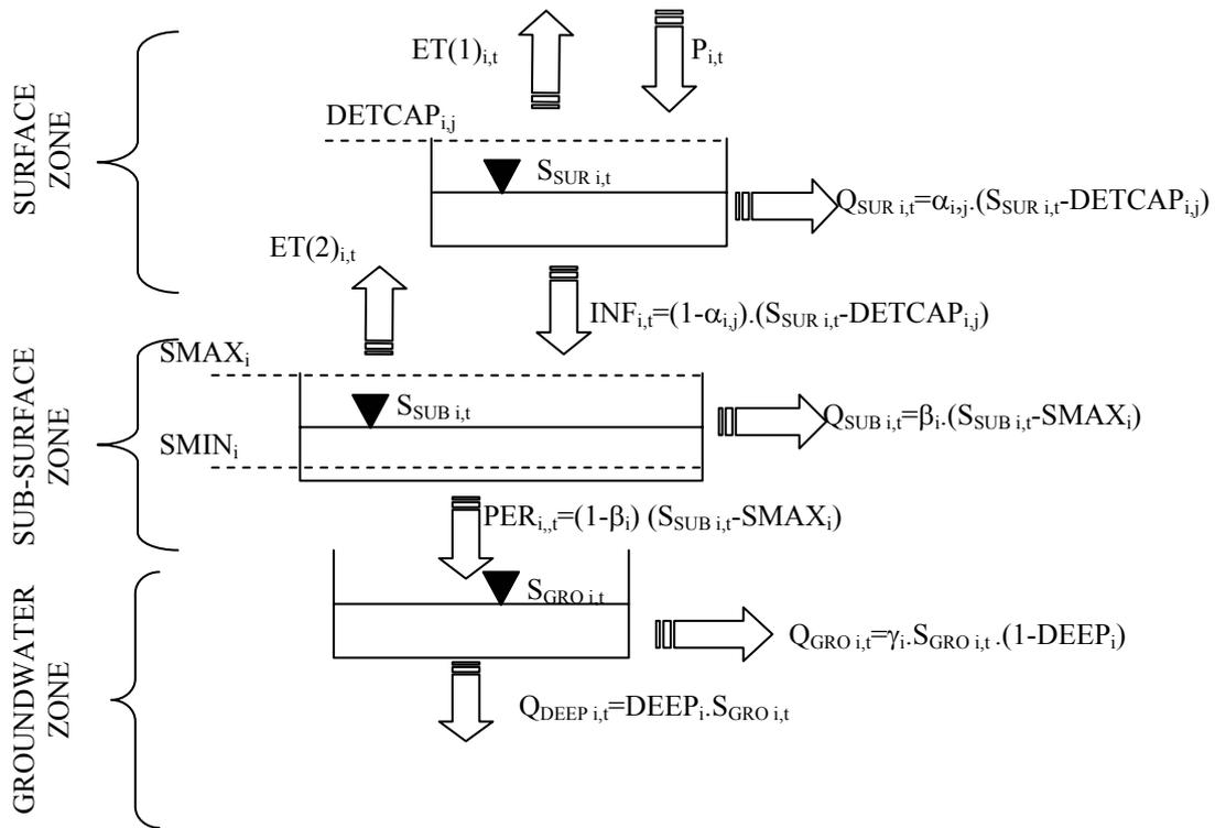
**Figure 1.** Vertical Water Budget Component of the DRRSM (ET: Evapotranspiration, P: Rainfall, DETCAP: Surface Detention Capacity, INF: Infiltration, PER: Percolation)
