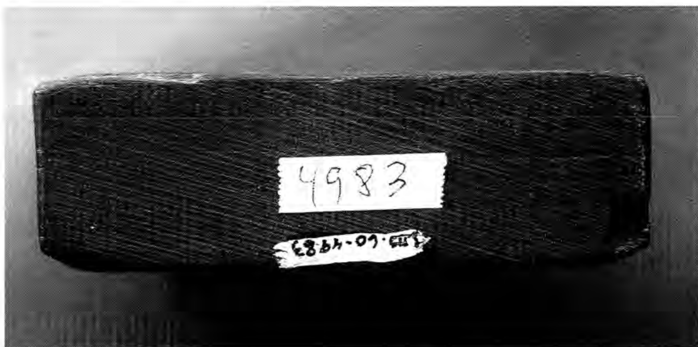
FIG. 13. Marks made by a saw. The equidistant marks on this slate artifact (LDS #60-4983) indicate it was cut by a modern saw.
