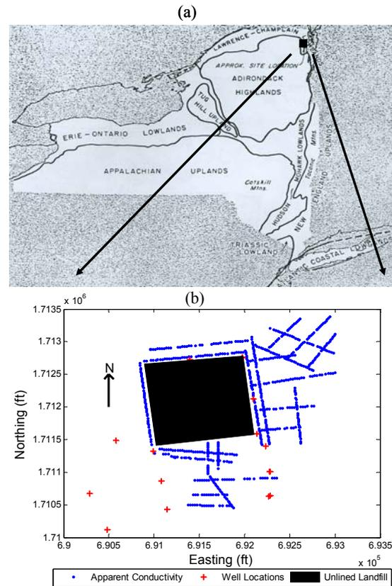
**Figure 1.** Location of (a) Schuyler Falls Landfill in upstate New York and (b) spatial representation of unlined landfill, available hydrochemistry well data and apparent conductivity data.
