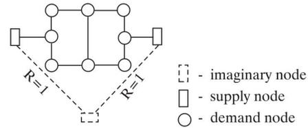
**Figure 3.** Imaginary node and imaginary links in network with more than one source node
