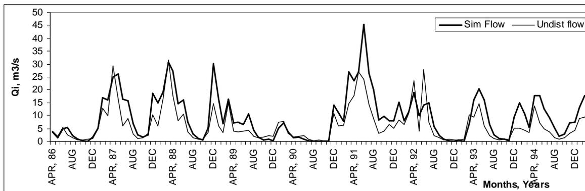
Figure 10. Comparison of simulated and undisturbed hydrographs of Zlatarishka catchment for the period 1986-1995
