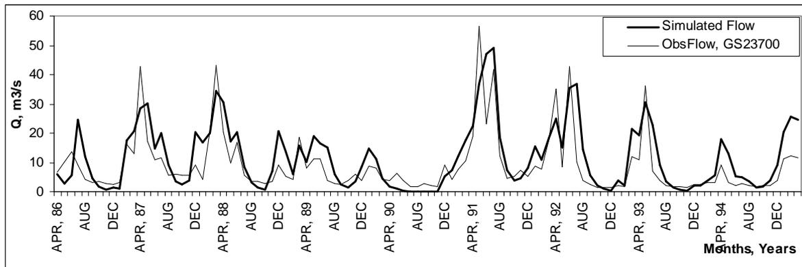
**Figure 3.** Calibration of BISTRA model for sub-basin Veliko Turnovo for the period 1986-1995
