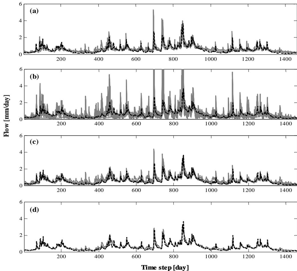
**Figure 2. Comparison of observed and simulated flow time-series from Oct 1984-Sept 1989 for the Thet at Bridgham.** (a) 90% confidence intervals derived using the regression, (b) ensemble of model results from using all 30 gauged catchment optimal models, (c) ensemble from using the optimal models of the 4 most similar gauged catchments, (d) the weighted average result of these 4 models.
