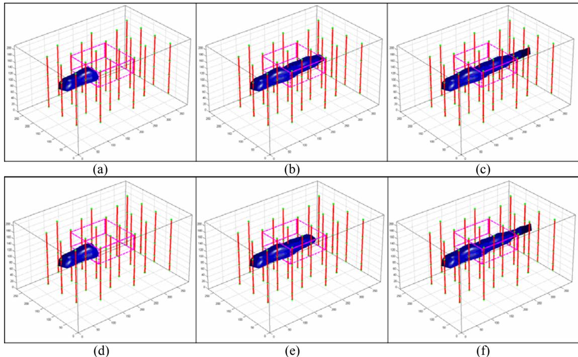
**Figure 3.** 3-D flow/transport model estimates of  $\text{NH}_4\text{Cl}$  (a) time=3 days, (b) time=8 days and (c) time=17 days; and 3-D ANN estimates of  $\text{NH}_4\text{Cl}$  at (d) time=3 days, (e) time=8 days and (f) time=17 days. The iso-contour indicates where normalized concentrations exceed 0.5.
