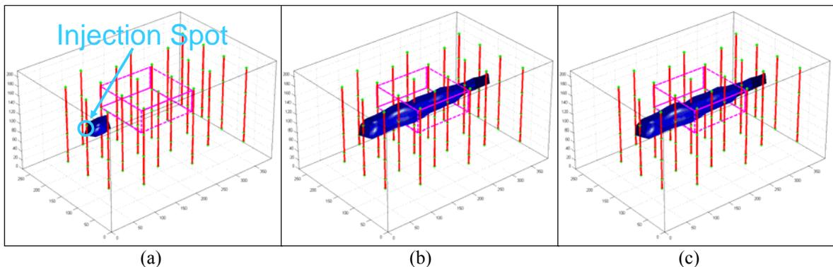
**Figure 4.** 3-D ANN estimates of  $\text{NH}_4\text{Cl}$  at (a) time=0 days and (b) time=19 days; and (c) flow/transport model prediction at time=19 days. The iso-contour indicates where normalized concentrations exceed 0.5.
