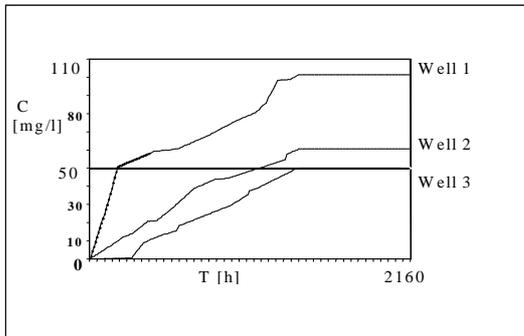
**Figure 3.** The pollutant concentration in the extracted water (maximum extraction case)
