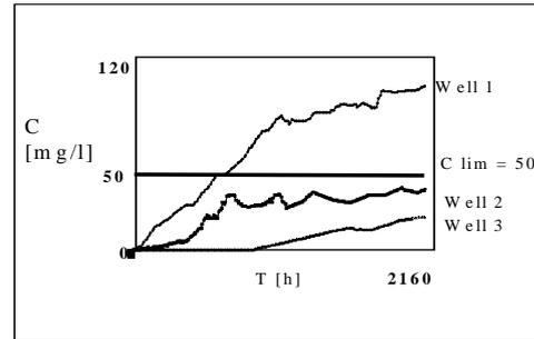
In Case 2, see Figure 2, no management policy can be applied, as, in order to satisfy the water demand, every well has to pump the maximum flow for the whole management horizon. Note that water pumped by well 1 overcomes the limit after 17 days, whereas, well 2 reaches such a limit after 60 days. Only well 3 can work over 3 months.
