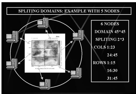
**Figure 3.** Cluster platform with 6 nodes for TEAP application.
