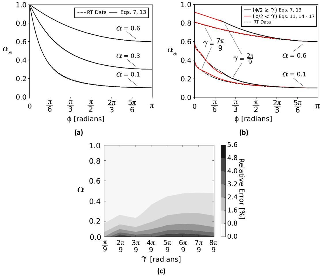
Figure 3. Apparent absorptivity for (a,b) full and (b) partial illumination. (c) Relative error for partial illumination averaged over cavity angle.
