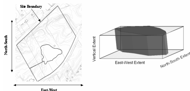
Figure 2. Incorporation of ArcGIS layers in site definition for both horizontal and vertical extent
