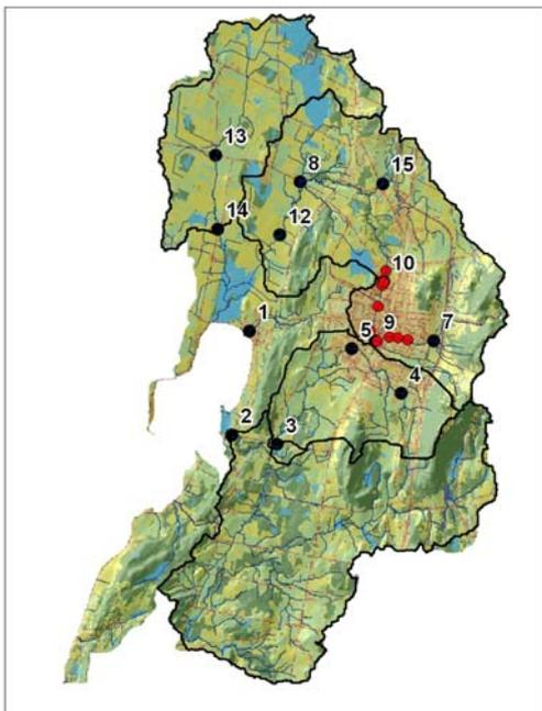
**Figure 1.** Monitoring points in the St. Albans watershed. Black points are in streams. Red points are stormwater outfalls. Agricultural sampling locations are not shown due to privacy restrictions. Landuse is illustrated using common colors of green for forest, red-orange for developed, yellow for agricultural, and blue for water/wetlands.
