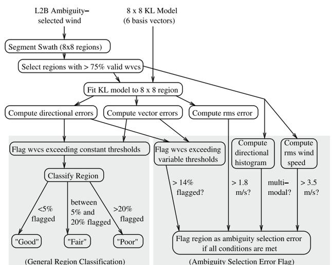
**Figure 4.** A flow diagram describing the QA analysis method. The left shaded box defines the region classification thresholds, and the right shaded box defines the thresholds involved with flagging a region as an ambiguity-selection error.
