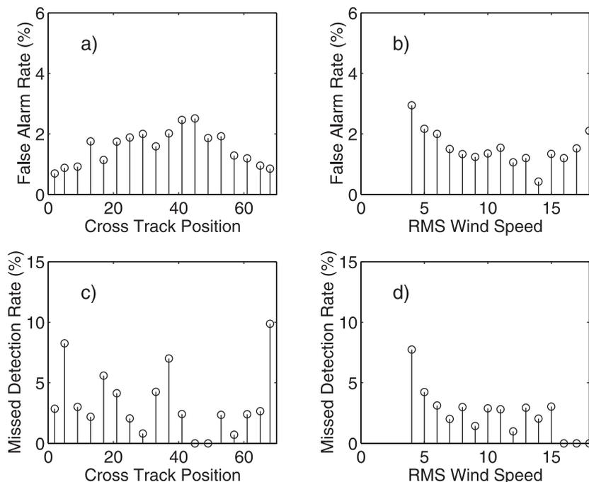
**Figure 6.** False alarm and missed detection rates for the ambiguity-selection error detection method per cross track and RMS wind speed. This data is taken from a test set of 15 subjectively analyzed revs.
