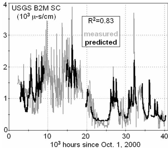
**Figure 7.** Measured and predicted marsh SC. Gaps mark missing input data. Marsh parameters are very
