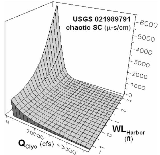
**Figure 8.** 3D response surface generated with a chaotic model of SC. The spikes in Figure 5 occur at low  $Q_{Clyo}$  and high  $WL_{Harbor}$ .
