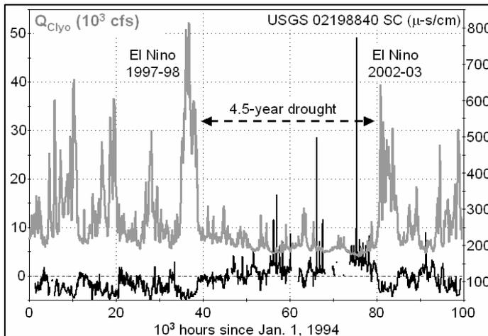
**Figure 2.** 11½ years of hourly  $Q_{Clyo}$  and SC at USGS 02198840, which was the farthest inland riverine gage. The SC spikes at center right occur at 28-day intervals, and are coincident peaking of the tidal range during the lowest flows of the drought.
