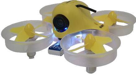
Fig. 6. Inductrix FPV aircraft used in test flights.
