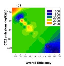
Figure 6: Pareto-optimal surface for the SOFC-PEM hybrid fuel Cell power Plant: (a) deterministic, (b) stochastic, (c) realistic
