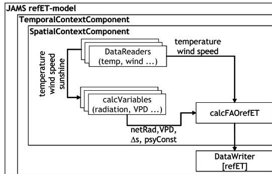
Figure 8: Graphical representation of the distributed JAMS-refET model
