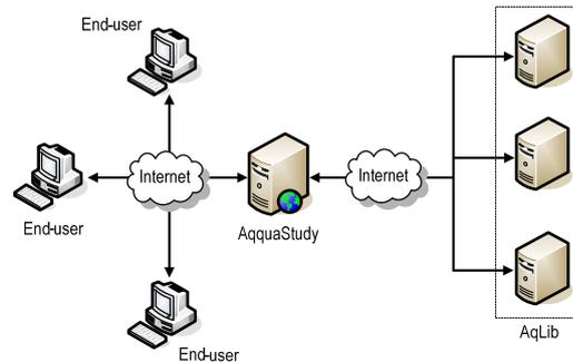
Figure 4. Hardware architecture of AqquaStudy
