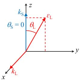
FIG. 3. A representation of the beam geometry used in our Yb measurements, following the notation of Ref. [24]. The laser beam travels in the *x* direction, represented by the red arrow labeled  $k_L$ . The scattered fluorescence signal is collected in the direction labeled by the blue arrow  $k_S$ . The polarization of the laser is represented by the red arrow labeled  $\epsilon_L$ . The angle between the laser polarization and vector pointing to the detector is represented by  $\theta_L$ .
