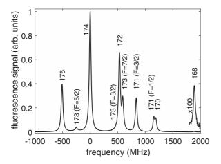
FIG. 2. Laser-induced fluorescence measurements of Yb atoms in the atomic beam. Zero frequency corresponds to the center of the <sup>174</sup>Yb transition. The different isotopes and upper state hyperfine levels are labeled in the plot.
