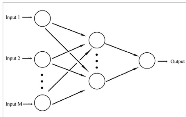
Figure 2. Principle Neural Network Structure
