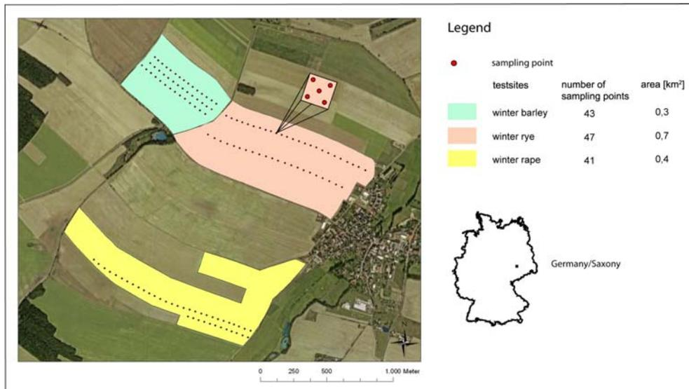
**Figure 1.** Testsites and schematic demonstration of the SSM sampling strategy (map source: Google Earth)
