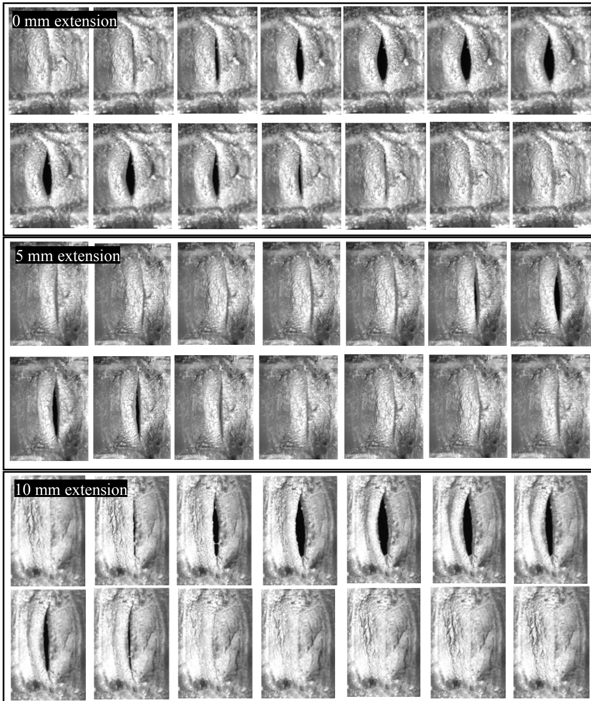
Figure 6. High-speed images taken during testing from a fiber vocal fold model at 0, 5, and 10 mm extensions.
