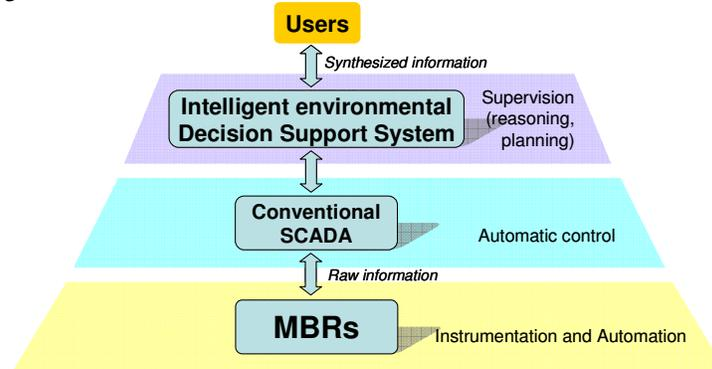
Figure 2. Hierarchical control architecture proposed for the integrated control of membrane bioreactors (adapted from [Ayesa et al., 2006]).
