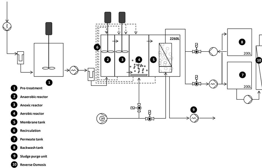
Figure 1. Schematic of the pilot plant under study.
