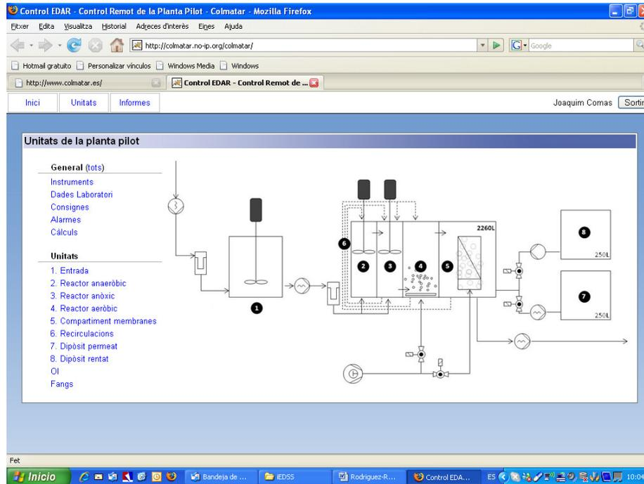
Figure 4. Homepage of the web-based IEDSS for membrane bioreactors.
