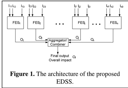
**Figure 1.** The architecture of the proposed EDSS.
