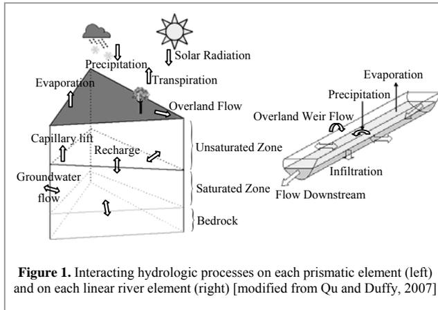
**Figure 1.** Interacting hydrologic processes on each prismatic element (left) and on each linear river element (right) [modified from Qu and Duffy, 2007]
