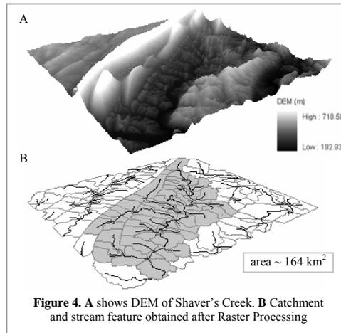
Figure 4. A shows DEM of Shaver's Creek. B Catchment and stream feature obtained after Raster Processing
