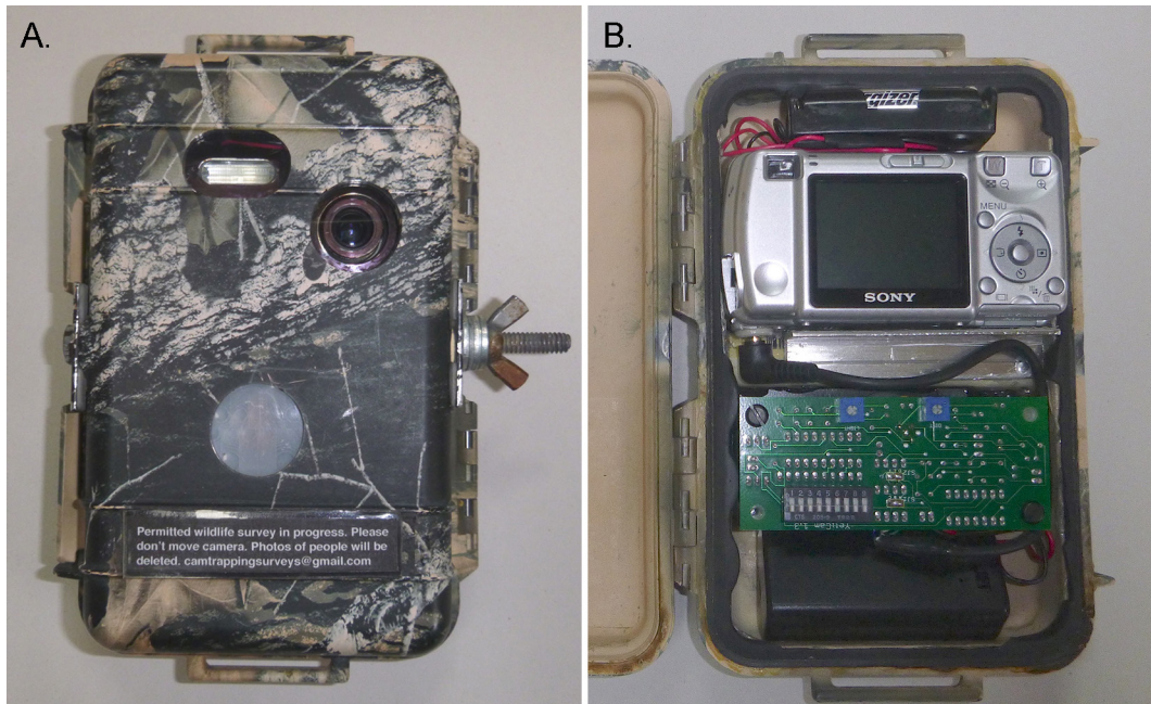
Fig. 2. Custom camera trap used for study. A , Closed camera trap showing sturdy exterior of case with lens, flash, and motion sensor. B , Case open to show camera, controller card with motion sensor, and add-on batteries for additional longevity.
