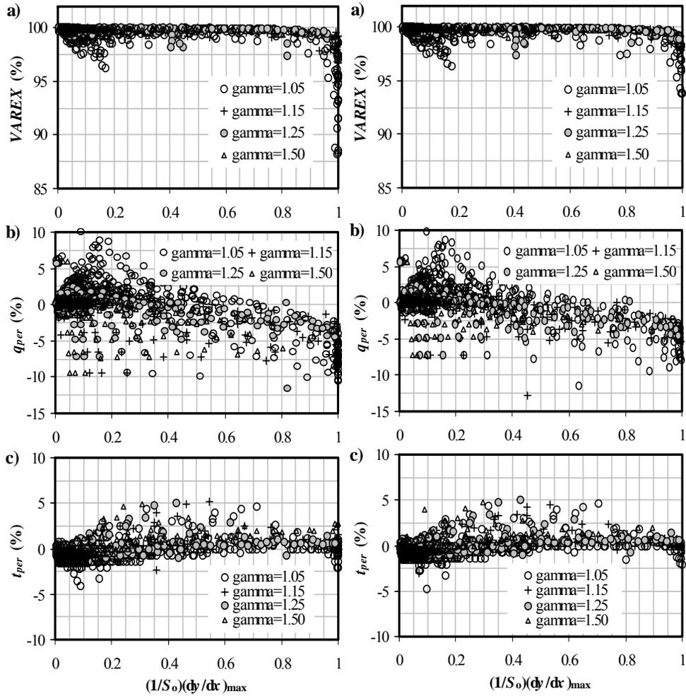
**Figure 3.** Error estimates of the multilinear diffusion model in comparison with the Saint-Venant's solutions for rectangular channel.
