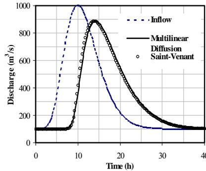
**Figure 2.** Hydrograph reproductions by the proposed multilinear diffusion and the Saint-Venant methods in a trapezoidal channel ( $S_o=0.0002$ ,  $n=0.02$ ,  $z=1.0$ ,  $I_b=100$  m<sup>3</sup>/s,  $I_p=1000$  m<sup>3</sup>/s,  $\gamma=1.15$ )
