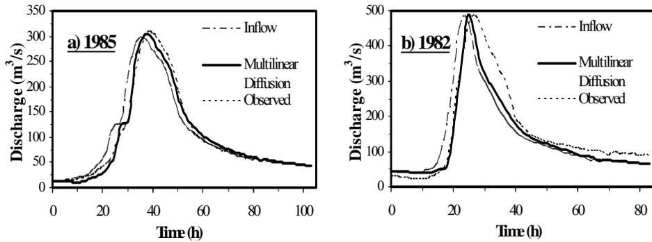
**Figure 5.** Typical flood routing simulations using the proposed method (Between Ponte Felcino and Torgiano sections of the Tiber River in Central Italy).
