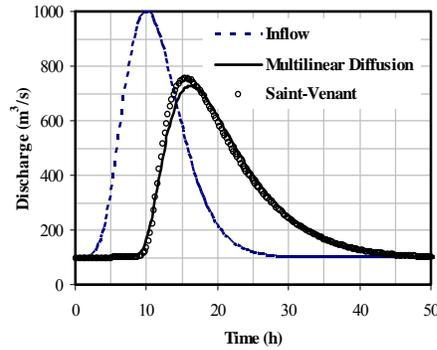
**Figure 1.** Hydrograph reproductions by the proposed multilinear diffusion and the Saint-Venant methods in rectangular channel ( $S_o=0.0002$ ,  $n=0.04$ ,  $I_b=100$  m<sup>3</sup>/s,  $I_p=1000$  m<sup>3</sup>/s,  $\gamma = 1.15$ )
