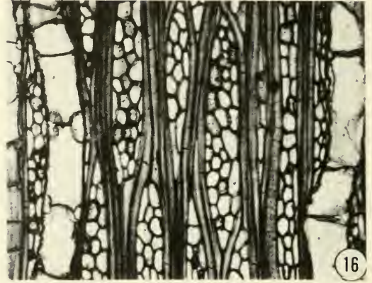
Fig. 16. Tangential section illustrating the heterocellular rays and septa in the fibretracheids (100X).
