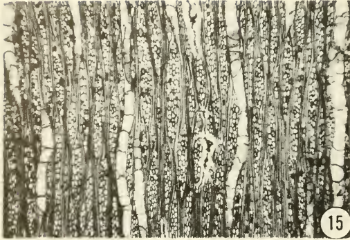
Fig. 15. Tangential section illustrating the relative size and distribution of multiseriate rays, fibretracheids, and vessels with tyloses (30X).
