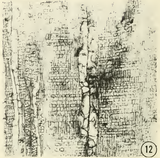
Fig. 12. Radial section illustrating the relative size and distribution of the vessels and cells of the heterocellular rays (33X).
