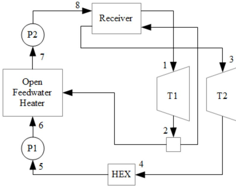
Fig. 4. Component schematic of steam Rankine cycle.
