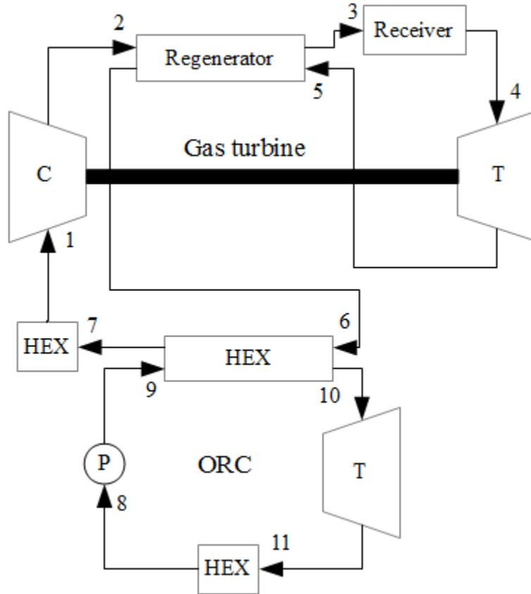
**Fig. 3. Component schematic of combined Brayton-Rankine cycle.**
