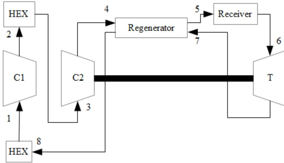
**Fig. 1. Component schematic of regenerative Brayton cycle.**
