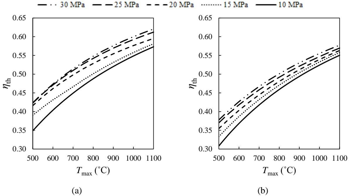
**Fig. 7. Thermal efficiency of the CO<sub>2</sub> recompression Brayton cycle as a function of maximum temperature for different maximum pressures under (a) wet-cooling and (b) dry-cooling conditions.**
