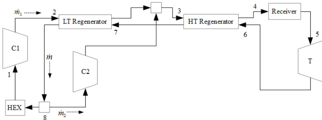
Fig. 2. Component schematic of recompression Brayton cycle.
