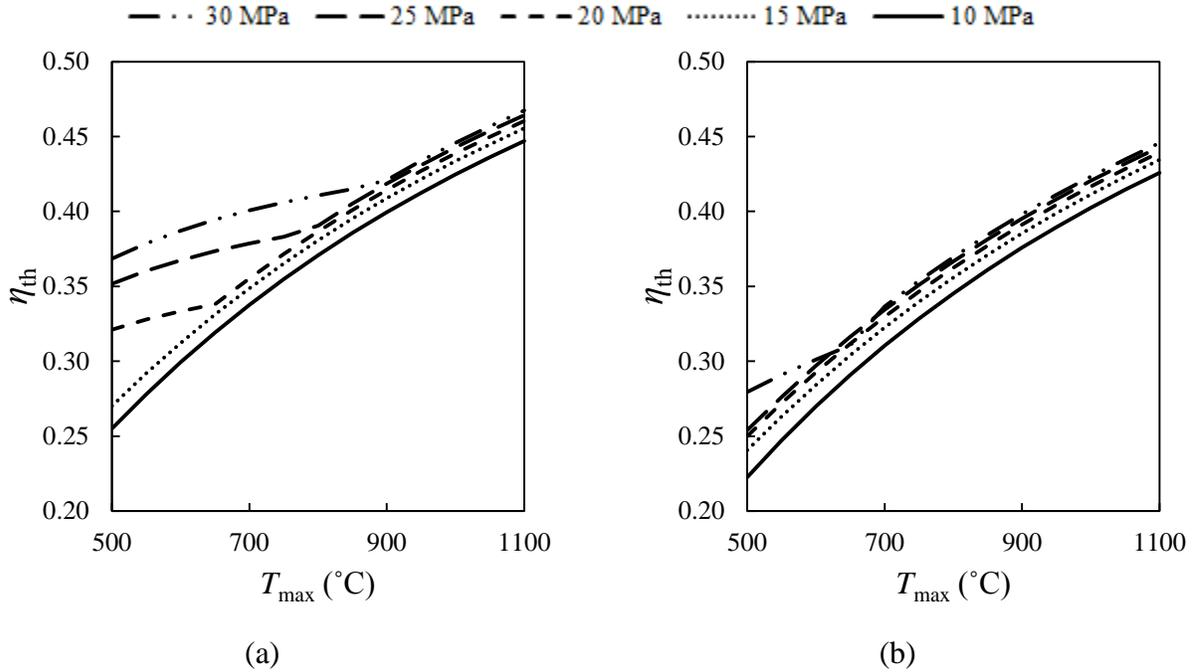
**Fig. 6. Thermal efficiency of the regenerated CO<sub>2</sub>-Brayton cycle as a function of maximum temperature for different maximum pressures under (a) wet-cooling and (b) dry-cooling conditions.**
