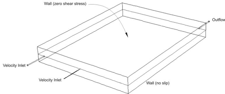
**Figure 3.** Boundary conditions defined for the rectangular tank
