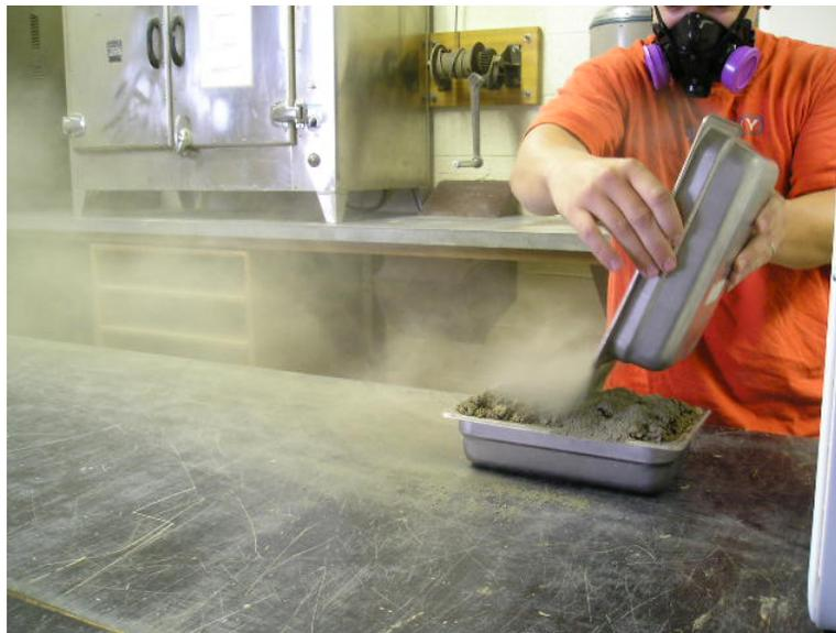
**Figure 3.1 Cement powder dispersion during blow test.**
