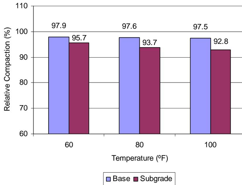
**Figure 4.12 Main effects of temperature on relative compaction.**
