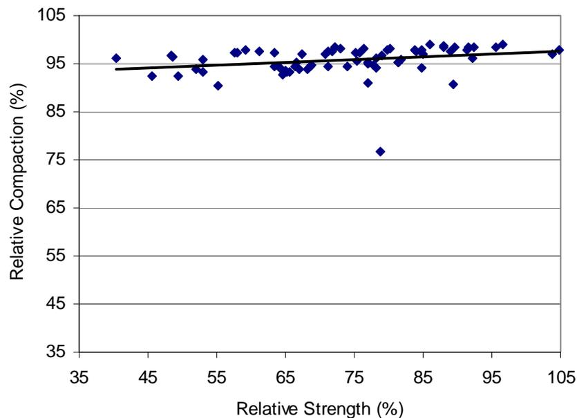
**Figure 4.15 Correlation between relative strength and relative compaction.**
