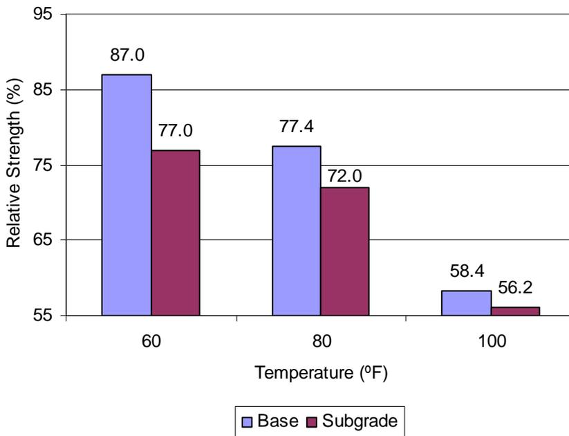
**Figure 4.6 Main effects of temperature on relative strength.**
