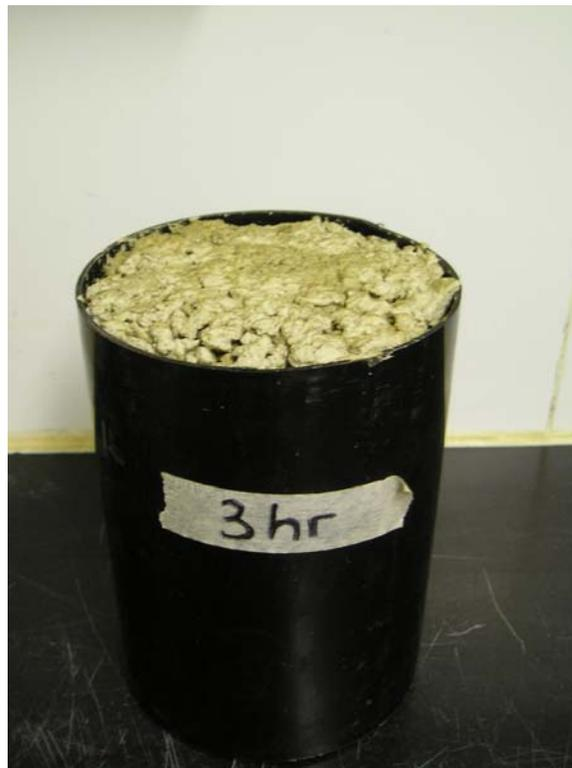
**Figure 3.2 Specimen of base material prepared for conditioning.**
