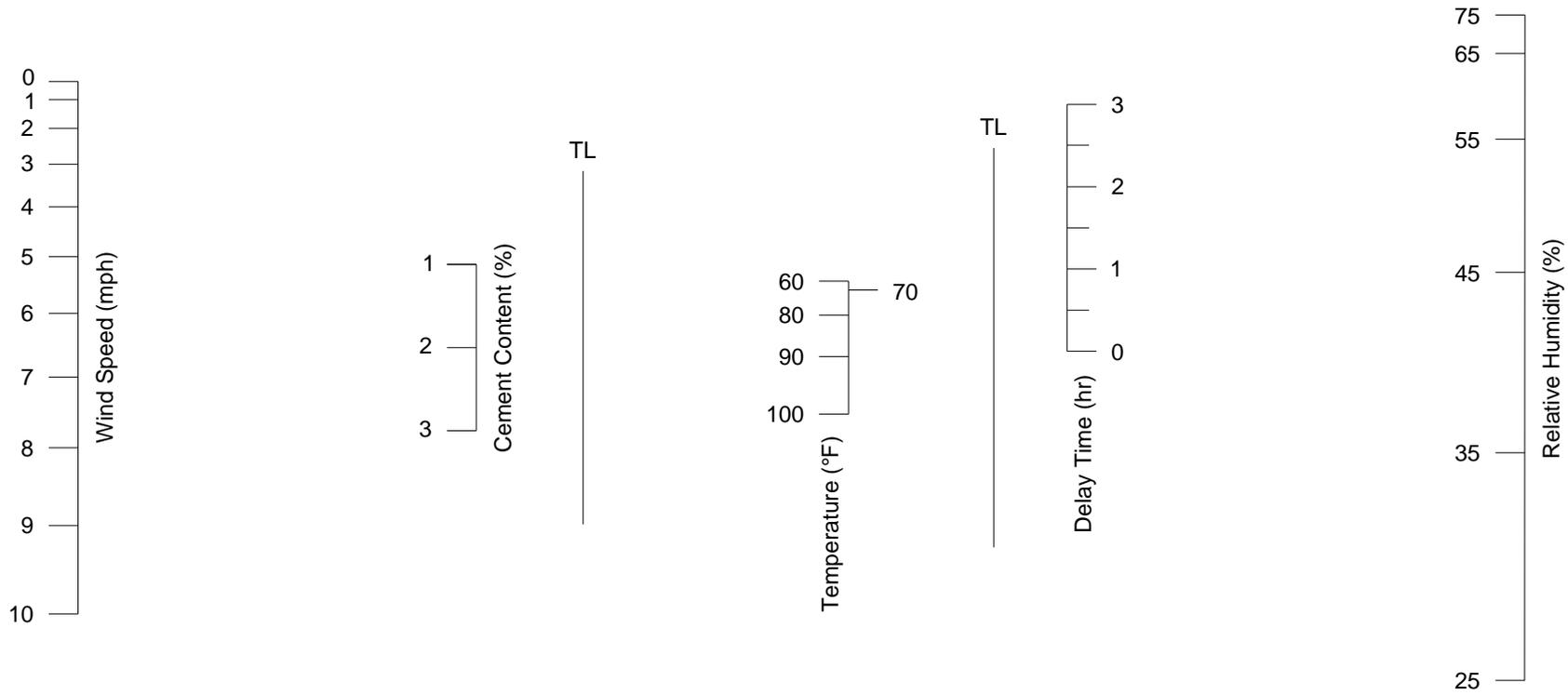
Figure 4.16 Base nomograph for minimum of 85 percent relative strength.
