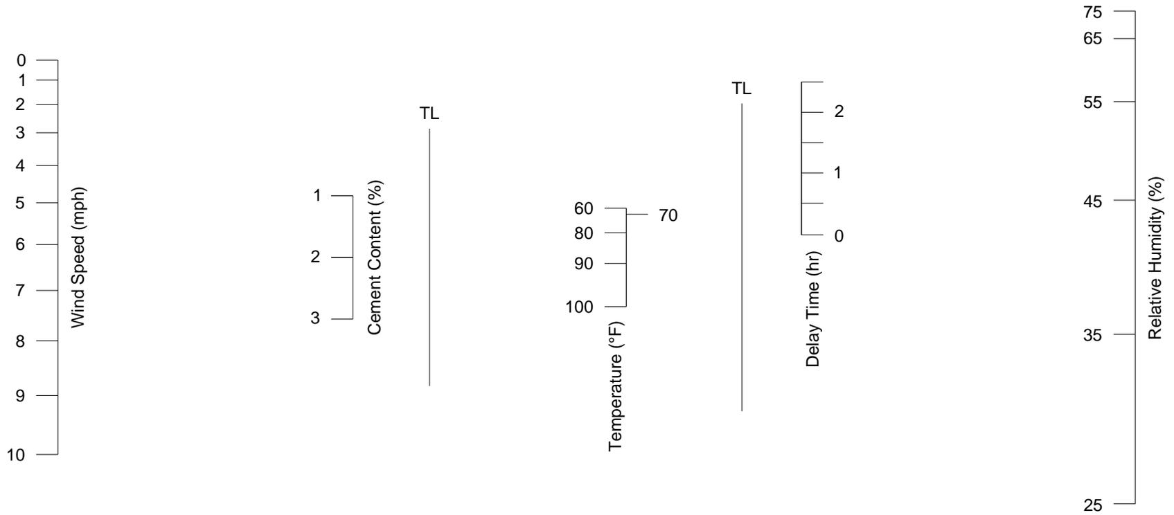
**Figure 4.17 Base nomograph for minimum of 90 percent relative strength.**
