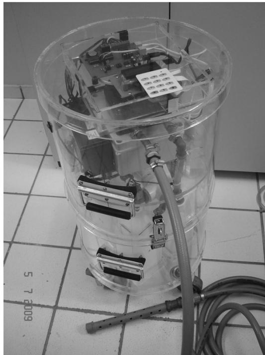
**Figure 1.** Front view of the automatic water sampler.
