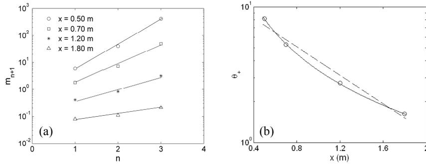
**Figure 2:** (a) Variation of center-line absolute moments with the moment order; (b) variation of ‘local’ concentration scale with downstream distances behind the point source, where the broken line is an exponential fit and the solid line is a power-law fit.
