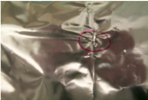
Hole in Bag Caused by Folding
