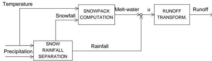
Figure 2: Hydrological model structure. Three sub-models are considered: “Snow-Rainfall separation”, “Snowpack computation” and “Runoff transformation”.
