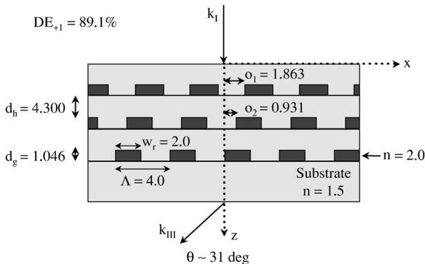
Fig. 8. Specifications for prototype design of a lidar scanner element.
