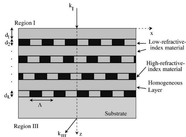
Fig. 1. Schematic illustration of the SVDOE structure.
