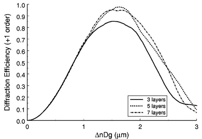
Fig. 3. Diffraction efficiency of a five-layer SVDOE as a function of total grating layer thickness ( $\Delta n = 0.1$ ).  $\lambda_0 = 2.06 \mu\text{m}$ ,  $\theta=9.885^\circ$ ,  $n_I = 1.5$ ,  $n_{III} = 1.5$ ,  $n_{\text{ridge}} = 1.6$ ,  $n_{\text{groove}} = 1.5$ ,  $d_{\text{homogeneous}} = 2.1 \mu\text{m}$ .
