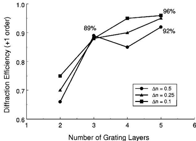
Fig. 7. Diffraction efficiency as a function of number of grating layers.  $\lambda_0 = 2.06 \mu\text{m}$ ,  $\theta = 0^\circ$ ,  $n_I = 1.5$ ,  $n_{III} = 1.5$ ,  $n_{\text{groove}} = 1.5$ . For  $\Delta n = 0.5$ ,  $n_{\text{ridge}} = 2.0$ ; for  $\Delta n = 0.25$ ,  $n_{\text{ridge}} = 1.75$ ; for  $\Delta n = 0.1$ ,  $n_{\text{ridge}} = 1.6$ .
