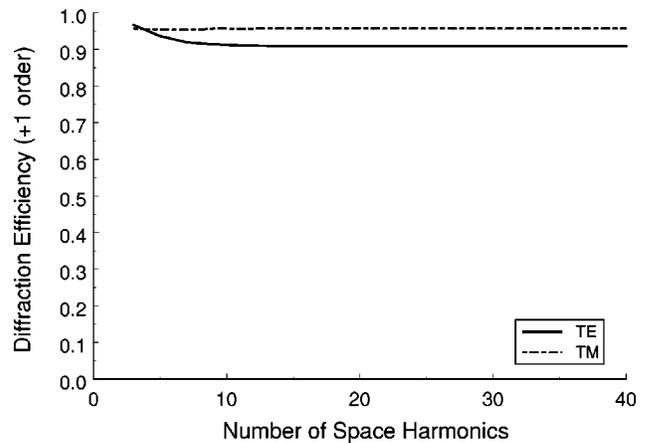
Fig. 2. Convergence of the diffraction efficiency as a function of the number of space harmonics retained in the calculation.  $\lambda_0 = 2.06 \mu\text{m}$ ,  $\theta=9.885^\circ$ ,  $n_I = 1.5$ ,  $n_{III} = 1.5$ ,  $n_{\text{ridge}} = 2.0$ ,  $n_{\text{groove}} = 1.5$ ,  $d_{\text{grating}} = 0.638$ ,  $d_{\text{homogeneous}} = 4.6 \mu\text{m}$ .
