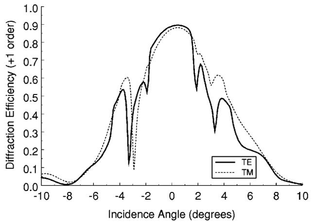
Fig. 9. Diffraction efficiency as a function of incidence angle for both TE and TM polarizations. Three grating layers,  $\lambda_0 = 2.06 \mu\text{m}$ ,  $\theta = 0^\circ$ ,  $n_I = 1.5$ ,  $n_{III} = 1.5$ ,  $n_{\text{ridge}} = 2.0$ ,  $n_{\text{groove}} = 1.5$ ,  $d_{\text{grating}} = 1.046 \mu\text{m}$ ,  $d_{\text{homogeneous}} = 4.300 \mu\text{m}$ .
