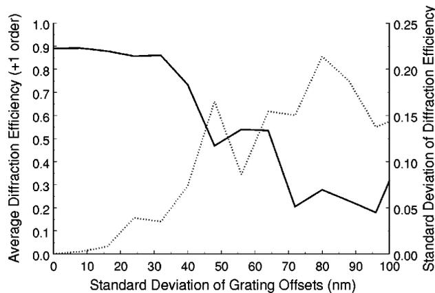
Fig. 11. Effect of statistical variation of grating layer offsets on the diffraction efficiency of the prototype lidar scanner. Three grating layers,  $\lambda_0 = 2.06 \mu\text{m}$ ,  $\theta = 0^\circ$ ,  $n_I = 1.5$ ,  $n_{III} = 1.5$ ,  $n_{\text{ridge}} = 2.0$ ,  $n_{\text{groove}} = 1.5$ ,  $d_{\text{grating}} = 1.046 \mu\text{m}$ ,  $d_{\text{homogeneous}} = 4.300 \mu\text{m}$ .
