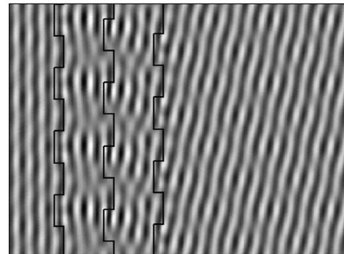
Fig. 10. RCWA representation of the electric field as it traverses the SVD OE prototype lidar scanner. Three grating layers,  $\lambda_0 = 2.06 \mu\text{m}$ ,  $\theta = 0^\circ$ ,  $n_I = 1.5$ ,  $n_{III} = 1.5$ ,  $n_{\text{ridge}} = 2.0$ ,  $n_{\text{groove}} = 1.5$ ,  $d_{\text{grating}} = 1.046 \mu\text{m}$ ,  $d_{\text{homogeneous}} = 4.300 \mu\text{m}$ .
