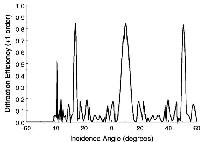
Fig. 6. Angular selectivity of a five-layer SVDOE with  $\Delta n = 0.5$ . Note that, for  $\theta_{\text{inc}} < -41^\circ$ , the +1 order is evanescent and hence the diffraction efficiency is zero.  $\lambda_0 = 2.06 \mu\text{m}$ ,  $n_I = 1.5$ ,  $n_{III} = 1.5$ ,  $n_{\text{ridge}} = 2.0$ ,  $n_{\text{groove}} = 1.5$ ,  $d_{\text{grating}} = 0.638 \mu\text{m}$ ,  $d_{\text{homogeneous}} = 4.9 \mu\text{m}$ .
