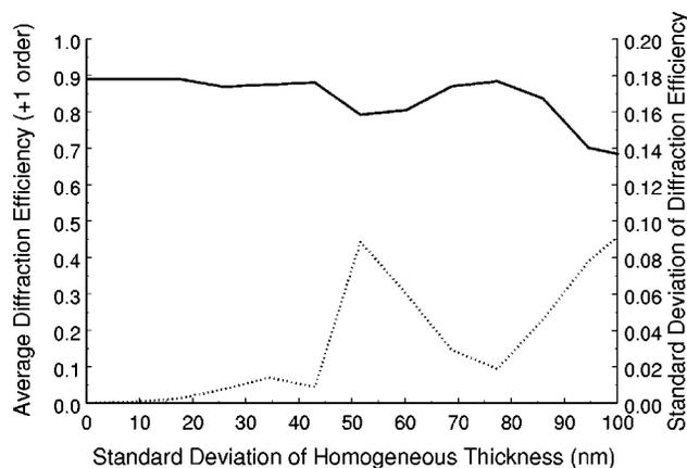
Fig. 12. Effect of statistical variation of homogeneous layer thickness on the diffraction efficiency of the prototype lidar scanner. Three grating layers,  $\lambda_0 = 2.06 \mu\text{m}$ ,  $\theta = 0^\circ$ ,  $n_I = 1.5$ ,  $n_{III} = 1.5$ ,  $n_{\text{ridge}} = 2.0$ ,  $n_{\text{groove}} = 1.5$ ,  $d_{\text{grating}} = 1.046 \mu\text{m}$ ,  $d_{\text{homogeneous}} = 4.300 \mu\text{m}$ .
