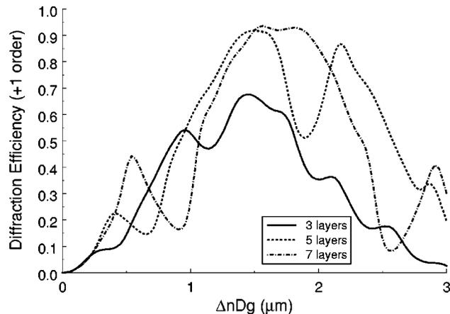
Fig. 4. Diffraction efficiency of a five-layer SVDOE as a function of total grating layer thickness ( $\Delta n = 0.5$ ).  $\lambda_0 = 2.06 \mu\text{m}$ ,  $\theta = 9.885^\circ$ ,  $n_I = 1.5$ ,  $n_{III} = 1.5$ ,  $n_{\text{ridge}} = 2.0$ ,  $n_{\text{groove}} = 1.5$ ,  $d_{\text{homogeneous}} = 4.6 \mu\text{m}$ .
