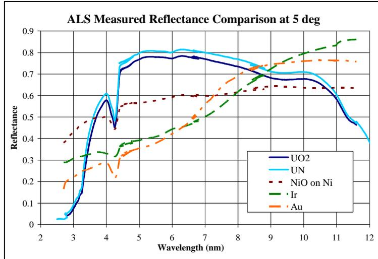
**Fig. 2: Measured reflectance of UO<sub>2</sub> from sample UO18, UN, NiO on Ni, Ir, and Au at 5° from 2.7 to 11.6 nm**
