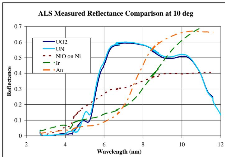
**Fig. 3: Measured reflectance of UO<sub>2</sub> from sample UO18, UN, NiO on Ni, Ir, and Au at 10° from 2.7 to 11.6 nm**
